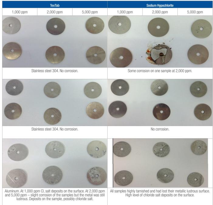
The pH of solutions varied little over the 30 day trial. pH of TexTabs solutions were ~6. pH of hypochlorite was 11-12. This higher pH causes corrosion of aluminum (Tables 2-3). The sample weights were unchanged over 30 days for TexTabs with only a very slight increase (0.40%) of one of the samples in 5,000 ppm (Tables 4-6). The weight change was much greater for aluminum in hypochlorite with weight gains in excess of 3% seen for some samples (Tables 7-9).
